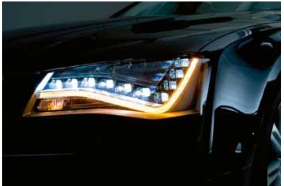
Figure 11: LED headlamp in the Audi A8 using Makrolon® LED2245 for low beams and daytime running lights
